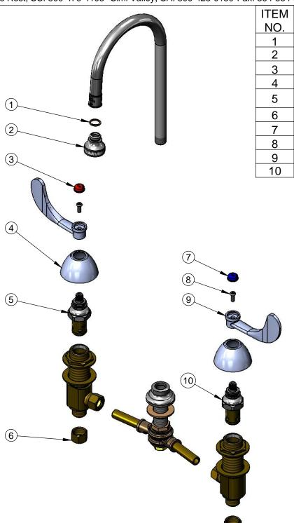
8" c/c Deck Mount Mixing Faucet w/ Eterna Cartridges, B-WH4 4" Wrist Action Handles, Rigid Gooseneck w/ B-0103 Rosespray
