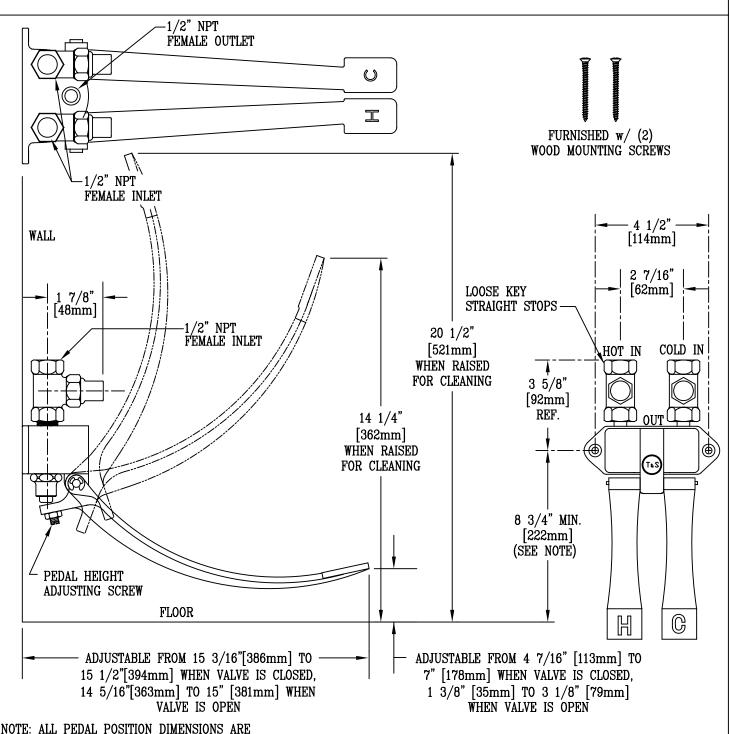
NOTE: ALL PEDAL POSITION DIMENSIONS ARE BASED ON MINIMUM RECOMMENDED MOUNTING HEIGHT OF 8 3/4" [222mm] ABOVE FINISHED FLOOR.
