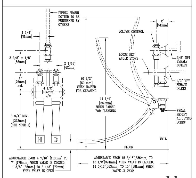
NOTE: ALL PEDAL POSITION DIMENSIONS ARE BASED ON MINIMUM RECOMMENDED MOUNTING HEIGHT OF 8 3/4" [222mm] ABOVE FINISHED FLOOR.
