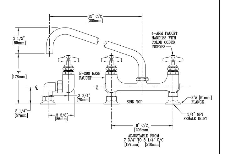
NOTE: DRILL 1 1/4"ø [32mm] HOLES ON 8"C/C IN SINK TOP.
