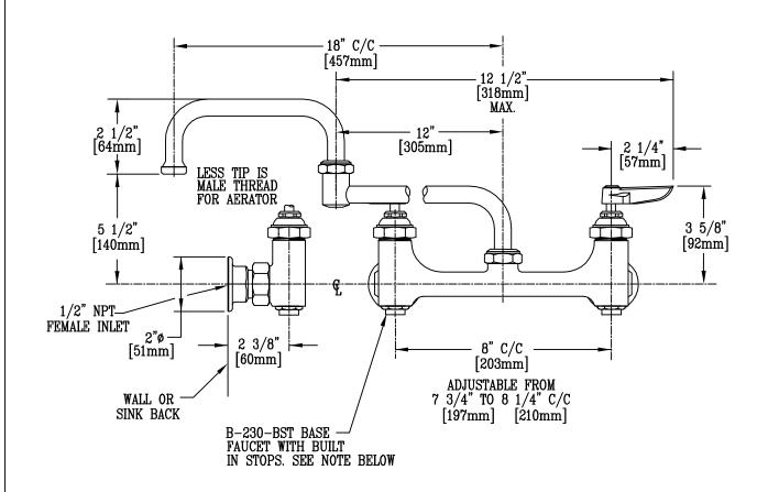
NOTE: PROVIDES INDIVIDUAL SHUT-OFF OF EACH VALVE WHEN MAINTENANCE IS REQUIRED.
