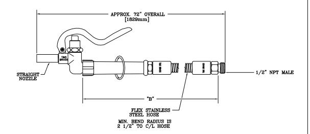
NOTE: "B" STANDARD HOSE UNIT IS 68"[1727mm] ANY LENGTH IS AVAILABLE FURNISHED W/ 1/2" MALE INLET NPT ADAPTER. ALSO AVAILABLE W/ 3/8",1/2" OR 3/4" NPT MALE OR FEMALE, AND GARDEN HOSE FEMALE ADAPTER.
