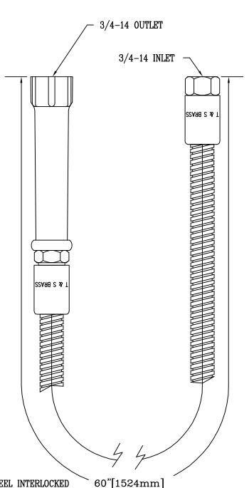
FLEXIBLE STAINLESS STEEL INTERLOCKED OUTER COVER WITH REINFORCED
