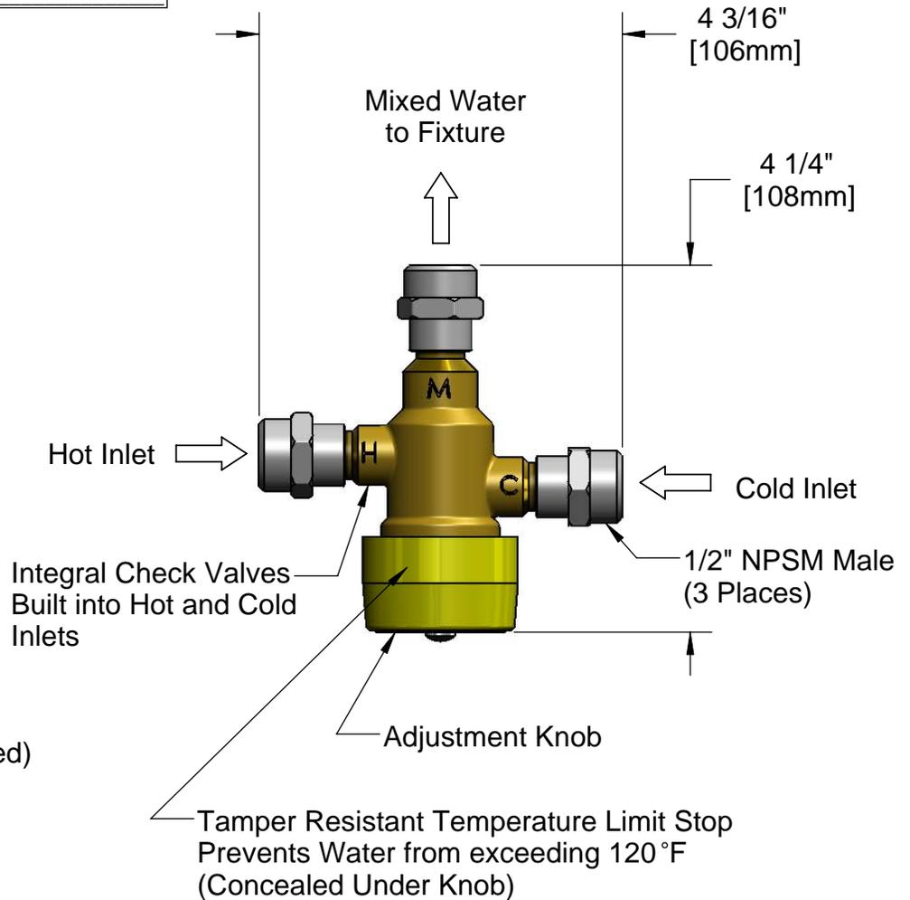
Note: This Valve is Tested and Certified to ASSE 1070 / ASSE 1016
