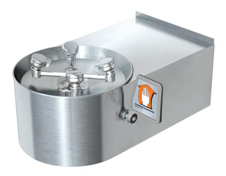
**APPLICATION:** WideArea<sup>™</sup> eye/face wash with vandal-resistant construction. Ideal for use in schools and other areas where equipment may be subject to abuse. All threaded connections are secured with set screws or cement to prevent disassembly.
