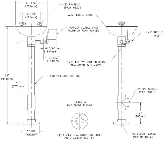
NOTE: EACH FS-PLUS SPRAY HEAD HAS A "FLIP-TOP" DUST COVER, INTERNAL FLOW CONTROL AND FILTER TO REMOVE IMPURITIES FROM THE WATER FLOW.
