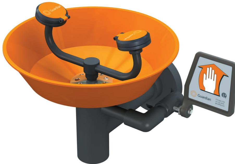
**APPLICATION:** Eye/face wash for wall mounting. Constructed entirely in PVC and PVC-coated brass. Ideal for use in industrial environments where harsh acids or caustics are present. Two large FS-Plus™ spray-type outlet heads deliver a flood of water for rinsing eyes and face.
