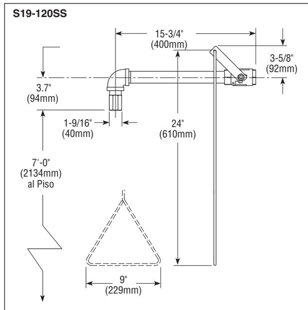
NOTE: All dimensions assume standard thread engagement. Variations in manufacturing allow for +/- 1/8" (3mm) per threaded joint. To find the tolerance of a dimension, add the number of thread joints in between a dimension and multiply it by 1/8" (3mm).
