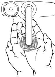
3. When hands are moved away from the "ON-Q" OPTIMA® Sensor, the loss of reflected light initiates an electrical signal that deactivates the Solenoid Valve, shutting off the water flow. The Circuit then automatically resets and is ready for the next user.
