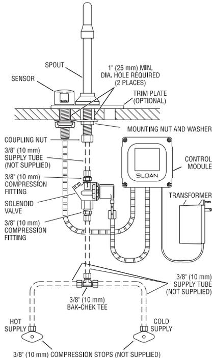
**ETF-770 Faucet with ADM Variation Mixing Valve for Hot and Cold Water Supply (shown with 4" trim plate)**
