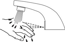
3. When hands are moved away from the OPTIMA® Sensor, the loss of reflected light initiates an electrical signal that deactivates the Solenoid Valve, shutting off the water flow. The Circuit then automatically resets and is ready for the next user.
