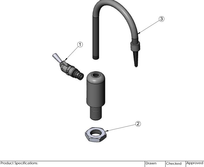
JRM Gray PVC Single Ledge Faucet w/ Rigid Gooseneck, Serrated Tip Outlet, & 3/8" NPT Female Inlet for Distilled or Deionzed Water Applications w/ Both Manual & Self-Closing Operations DMH JHB Scale: Date: NTS 07/08/09
