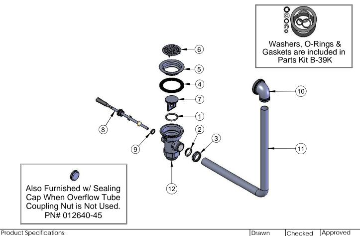
Waste Drain Valve w/ Lever Handle, 3" Sink Opening, 2" NPT Male Outlet, 1 1/2" NPT Male Adapter & Overflow Tube w/ Head Asm.
