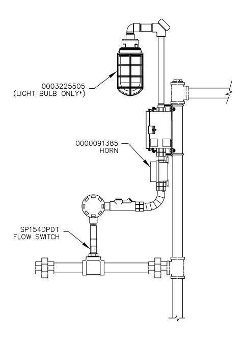
\* TEMPERATURE CODE IS AFFECTED BY BULB WATTAGE. RECOMMENDED 60 WATT BULB YIELDS T2C (230 DEG C), 150 WATT YIELDS T2 (300 DEG C).
