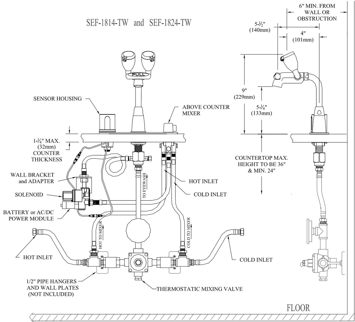
**SEF-1814-TW** -8" Sensorflow, eyewash faucet, ACM, battery and Thermostatic Valve for Eyewash
