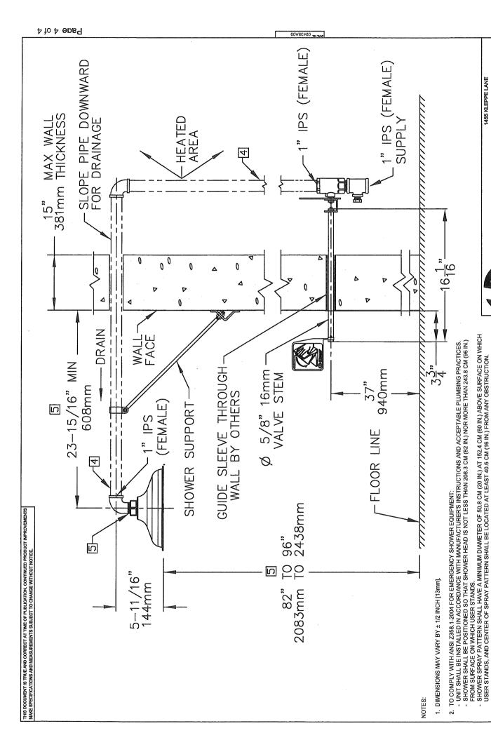
HAWS® and other trademarks used in these materials are the exclusive property of Haws Corporation. STATE OF THE PROPER SHOWER STATES OF THE STA 5 DO NOT USE REGULAR PIPE SEALANT. IF NECESSARY USE DOW CORNING 832 SEALANT PLACING 5 SMALL BEADS ON THE MALE THREADS, JUST ABOVE THE FIRST THREAD. ©2009 Haws Corporation - All Rights Reserved
