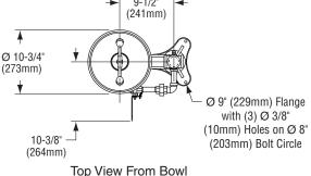
NOTE: All dimensions assume standard thread engagement. Variations in manufacturing allow for +/- 1/8" (3mm) per threaded joint. To find the tolerance of a dimension, add the number of thread joints in between a dimension and multiply it by 1/8" (3mm).
