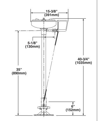
NOTE: All dimensions assume standard thread engagement. Variations in manufacturing allow for +/- 1/8" (3mm) per threaded joint. To find the tolerance of a dimension, add the number of thread joints in between a dimension and multiply it by 1/8" (3mm).
