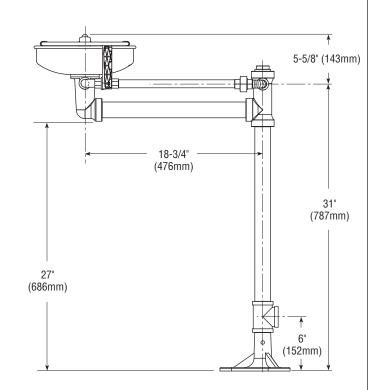
NOTE: All dimensions assume standard thread engagement. Variations in manufacturing allow for +/- 1/8" (3mm) per threaded joint. To find the tolerance of a dimension, add the number of thread joints in between a dimension and multiply it by 1/8" (3mm).
