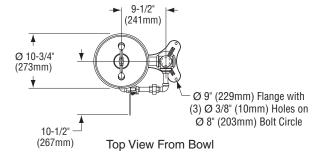
NOTE: All dimensions assume standard thread engagement. Variations in manufacturing allow for +/- 1/8 (3mm) per threaded joint. To find the tolerance of a dimension, add the number of thread joints in between a dimension and multiply it by 1/8 (3mm).
