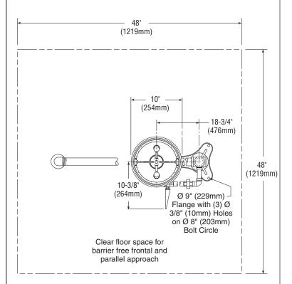
NOTE: All dimensions assume standard thread engagement. Variations in manufacturing allow for +/- 1/8" (3mm) per threaded joint. To find the tolerance of a dimension, add the number of thread joints in between a dimension and multiply it by 1/8" (3mm).
