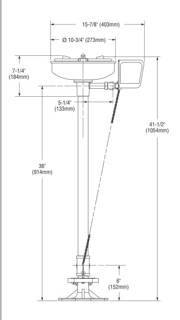
NOTE: All dimensions assume standard thread engagement. Variations in manufacturing allow for +/- 1/8" (3mm) per threaded joint. To find the tolerance of a dimension, add the number of thread joints in between a dimension and multiply it by 1/8" (3mm).
