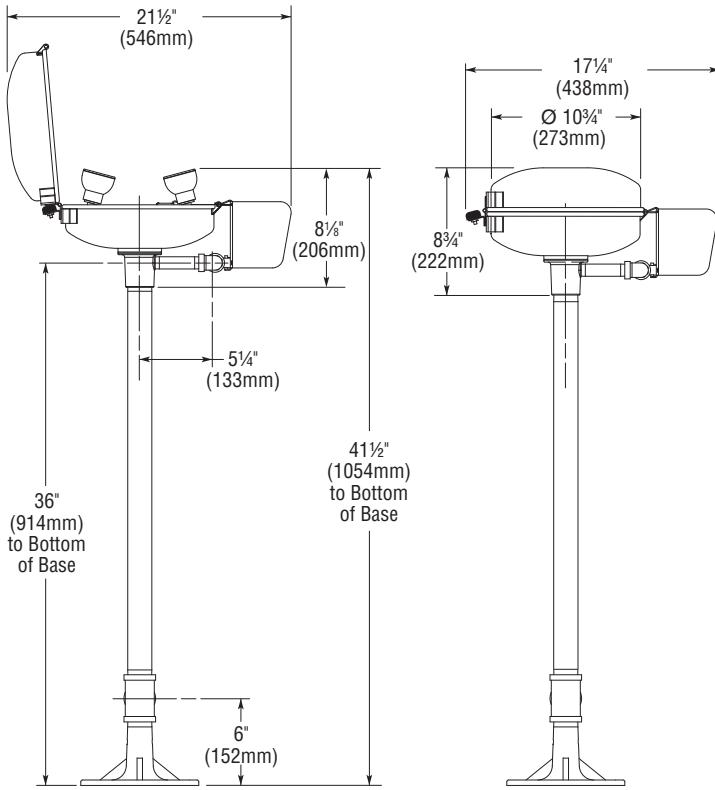
**NOTE:** All dimensions assume standard thread engagement. Variations in manufacturing allow for +/-  $\frac{1}{8}$ " (3mm) per threaded joint. To find the tolerance of a dimension, add the number of thread joints in between a dimension and multiply it by  $\frac{1}{8}$ " (3mm).
