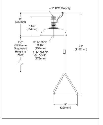
2. To assemble the pull rod, thread jam nut on to threaded end, then thread pull rod into coupling as shown. Tighten jam nut.
