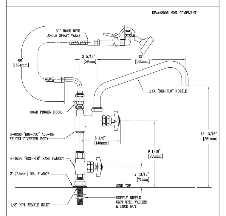
NOTE: DRILL 1 1/4" [32mm] HOLE ON 8"C/C IN SINK TOP.
