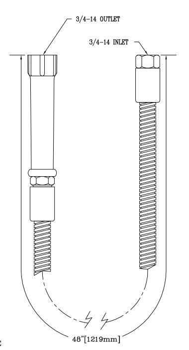
FLEX STAINLESS STEEL HOSE WITH POLYURETHANE INNER HOSE
