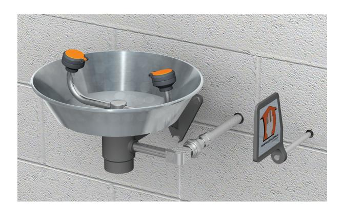
**APPLICATION:** Freeze-resistant eyewash for wall mounting. Valve and supply line are located behind wall in heated area to prevent freezing. Self-draining valve permits water to drain completely from unit after use. Since unit is intended for use in cold weather conditions, consideration should be given to supplying unit with tempered water in accordance with ANSI Z358.1-2004. See "Tempering Units" section for more information.
