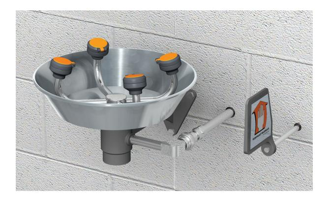
**APPLICATION:** Freeze-resistant WideArea<sup>™</sup> eye/face wash for wall mounting. Valve and supply line are located behind wall in heated area to prevent freezing. Self-draining valve permits water to drain completely from unit after use. Since unit is intended for use in cold weather conditions, consideration should be given to supplying unit with tempered water in accordance with ANSI Z358.1-2004. See "Tempering Units" section for more information.
