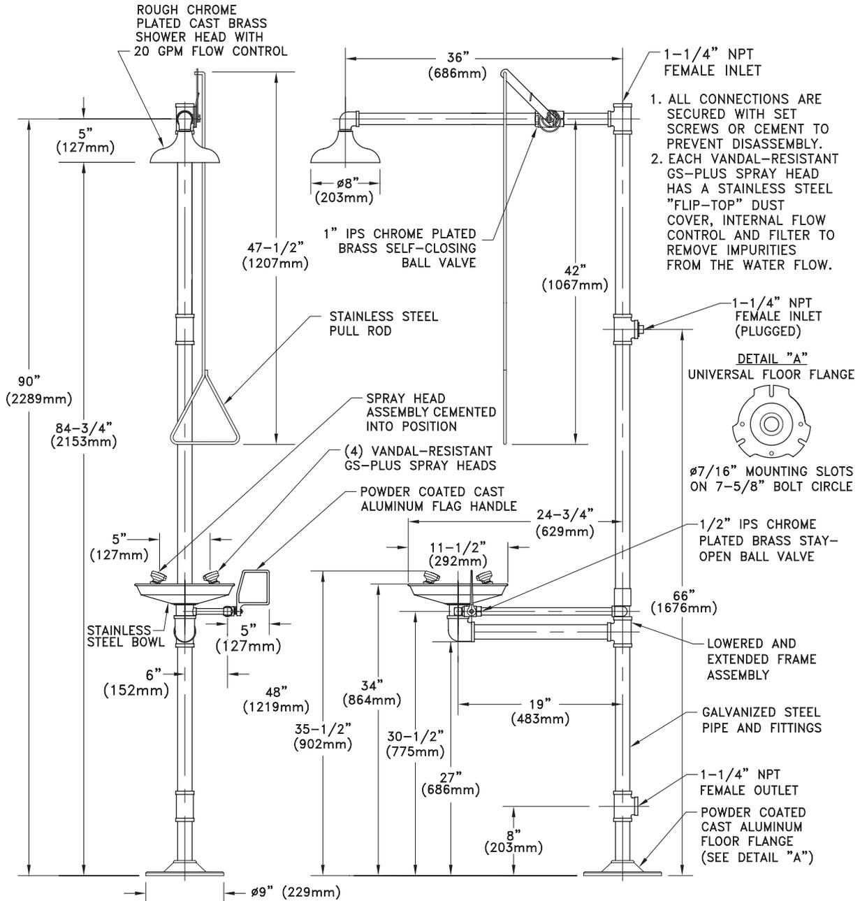
1. ALL CONNECTIONS ARE SECURED WITH SET SCREWS OR CEMENT TO PREVENT DISASSEMBLY.
