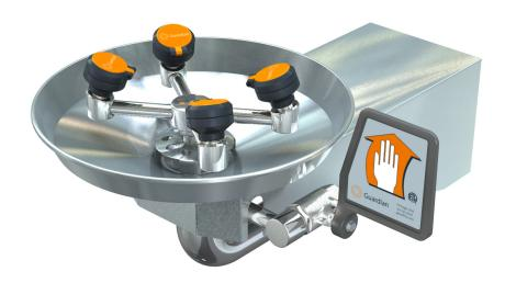
**APPLICATION:** Handicapped accessible WideArea™ eye/face wash for wall mounting. Bowl is lowered and extended to permit access by wheelchair user. Profile of unit is "flattened" to comply with maximum height and knee clearance requirements.
