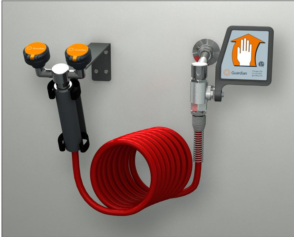
**APPLICATION:** Dual purpose eyewash/drench hose for wall mounting. Unit meets the provisions of ANSI Z358.1 - 2004 as both an eyewash and a drench hose. Unit may be left in the mounting bracket for use as a fixed eyewash, leaving user's hands free. Alternatively, unit may be removed for use as a drench hose to rinse any part of user's eyes, face or body.
