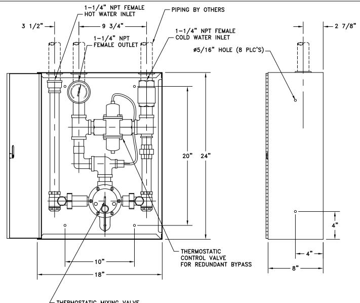
THERMOSTATIC MIXING VALVE \* LOCKING TYPE TEMPERATURE REGULATOR
