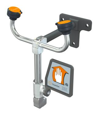
**APPLICATION:** Eyewash for wall mounting. Two GS-Plus™ spray-type spray heads deliver a flood of water for rinsing eyes. Unit is provided without bowl or drain for waste water. Note: Floor drain should be provided underneath unit to prevent accumulation of water on floor.
