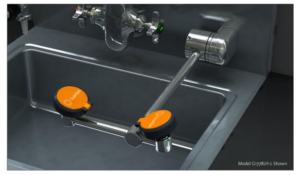
**APPLICATION:** AutoFlow<sup>™</sup> eye/face wash for mounting on wall. Spray heads swing down from storage to operational position, activating water flow. Available in a variety of spray head configurations to minimize obstructions at a sink. *Note: If unit is not installed at a sink, floor drain should be provided underneath unit to prevent accumulation of water on floor.*
