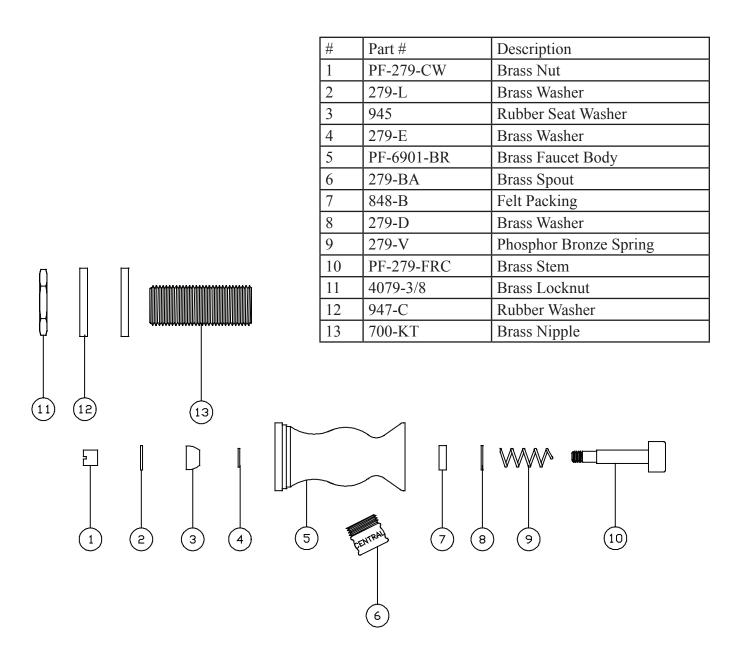
The parts listed in the parts breakdown above may not be offered separately as replacement parts. Please review the Replacement Parts page for the authorized replacement parts that are available for this item.
